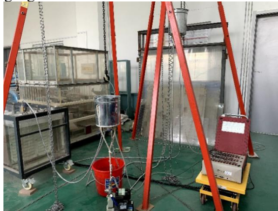
Figure 1: Sand box model test device.
